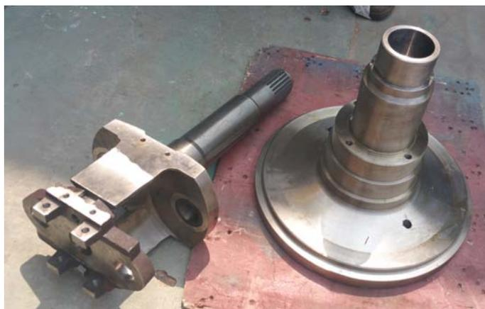
Main shaft and hollow shaft
